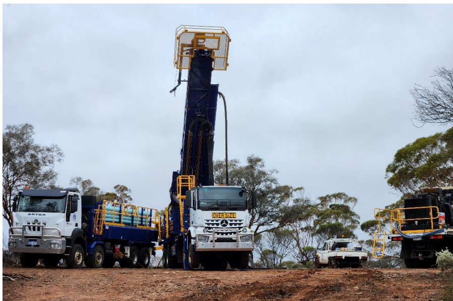
Figure 1: RC rig drilling at the Big Red Extension target
