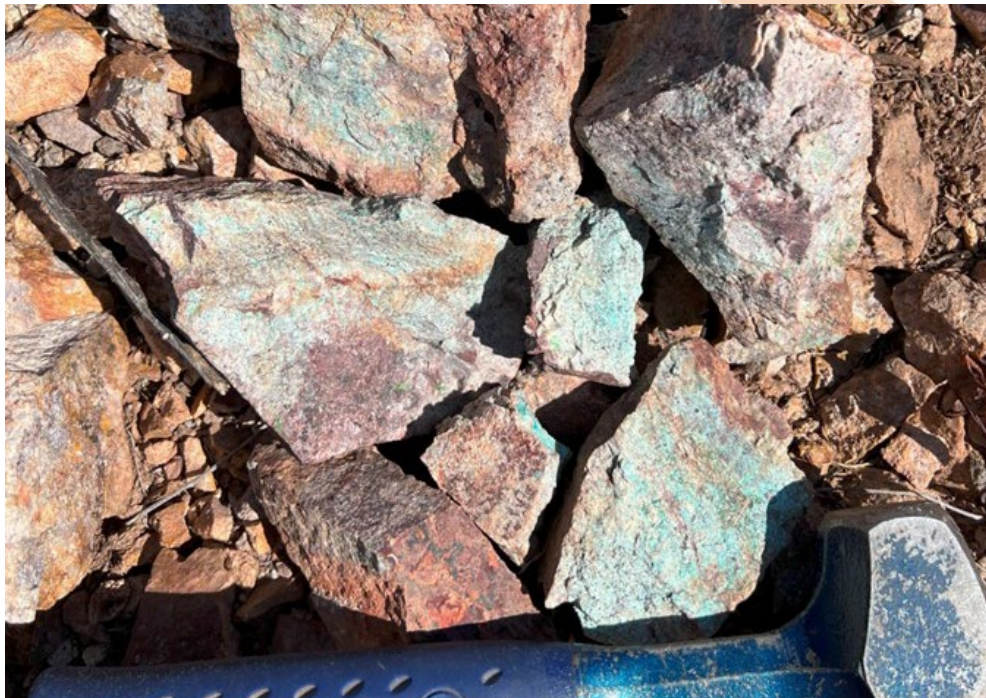
Figure 3: Sun Devil prospect sample DC0107 - 30,800 ppm (3.08%) Cu & 58 ppm Mo. Highly weathered ?Proterozoic intrusive rock with stockwork veining and supergene chrysocolla overprint.
