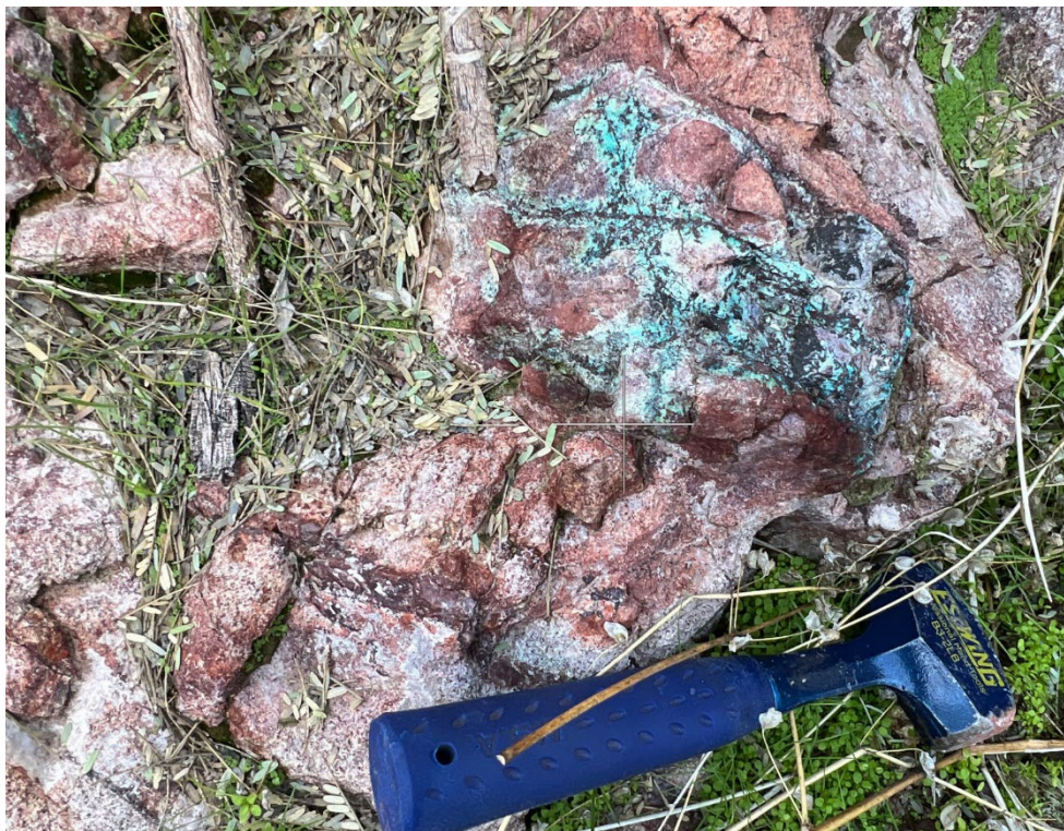
Figure 4: Sun Devil prospect sample DC0200 - 11,150 ppm (1.15%) Cu & 156 ppm Mo. Exposure in wall of valley, stockwork, early veins with k-feldspar with later quartz + Fe-Ox veins with k-feldspar selvages, supergene chrysocolla overprint.
