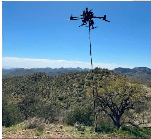
Figure 5: Drone magnetic surveys underway at the Copper Wolf Project.
