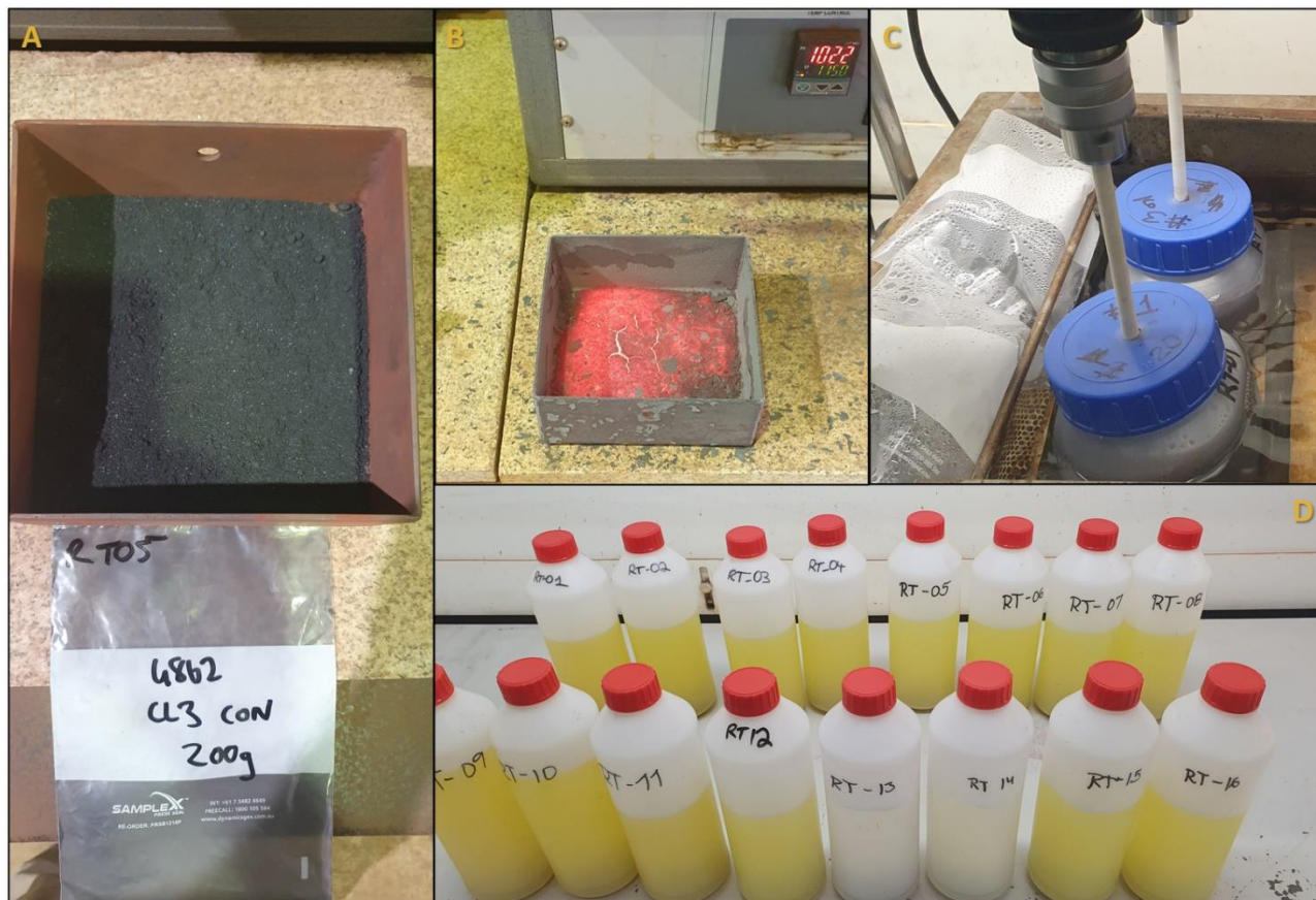
Figure 2; Photos showing A) Magnetic concentrate prior to roasting, B) Sample removed from oven after roasting, C) Water leaching from roasted sample & D) Filtered liquor containing leached Vanadium.
