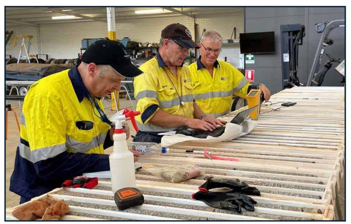
Figure 5: Some members of GSM technical team logging Eucla diamond drill core.
