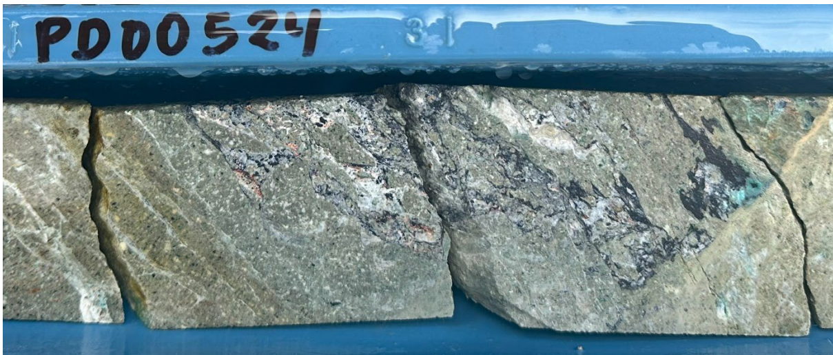
Figure 4: Example of copper mineralisation (chalcocite) at around 82.45m depth at Cumbre Coya Target (23PCCD0002)
