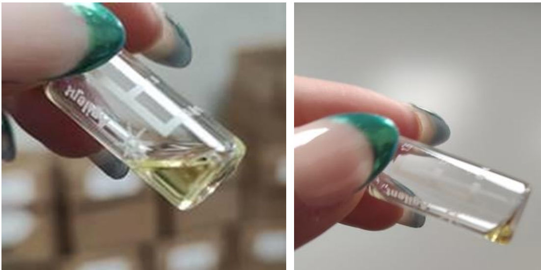
Figure 1 - Condensate recovered from flashed downhole reservoir fluid samples from Mukuyu-2 / ST1 well from Upper Angwa (on left) and Lower Angwa formations (on right) with API gravity of 50-60
