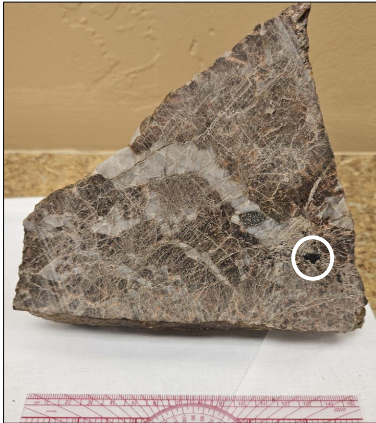
Photo 1 – Field sample of brecciated pegmatite collected from the Silver Dollar mine. Note the quartz veins and unknown opaque black mineral grain (circled white). This localised 1cm x 1cm area returned a pXRF reading of 2,170ppm U_3O_8 and 23,114 ppm ThO_2 (spot pXRF reading ID 1108).
