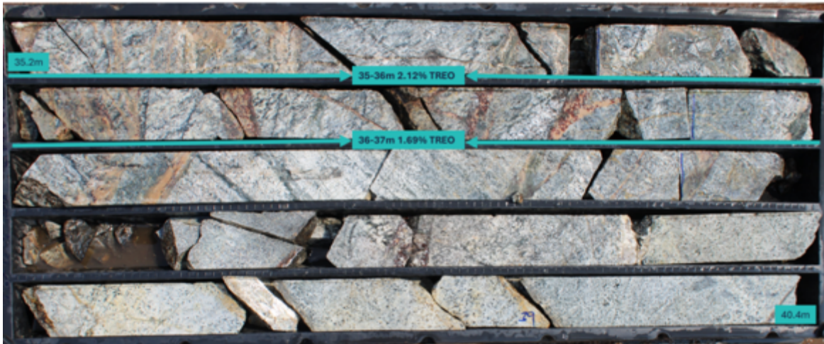
Figure 4. Half drill core of MDD007 showing high-grade rare earth mineralisation in the Machinga deposit.
