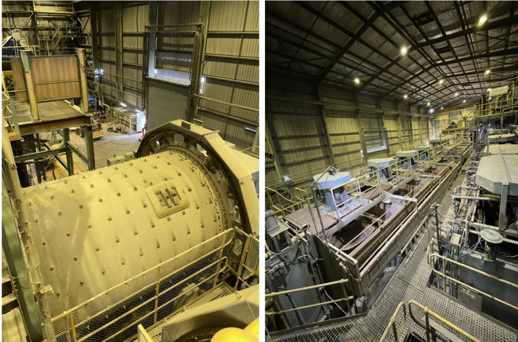
Figure 5: Ball mill and rougher/cleaner/scavenger units in mill.
