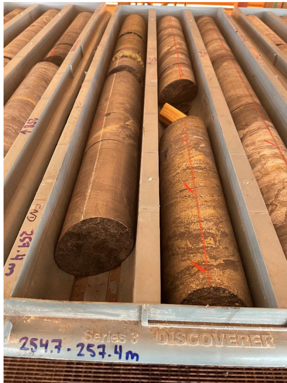
Figure 2-3: 23NFRCDM002 diamond drilled core, ~250m depth
