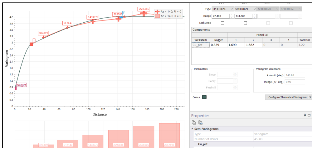
Figure 4-7: FWS Directional variogram, 140° azimuth
