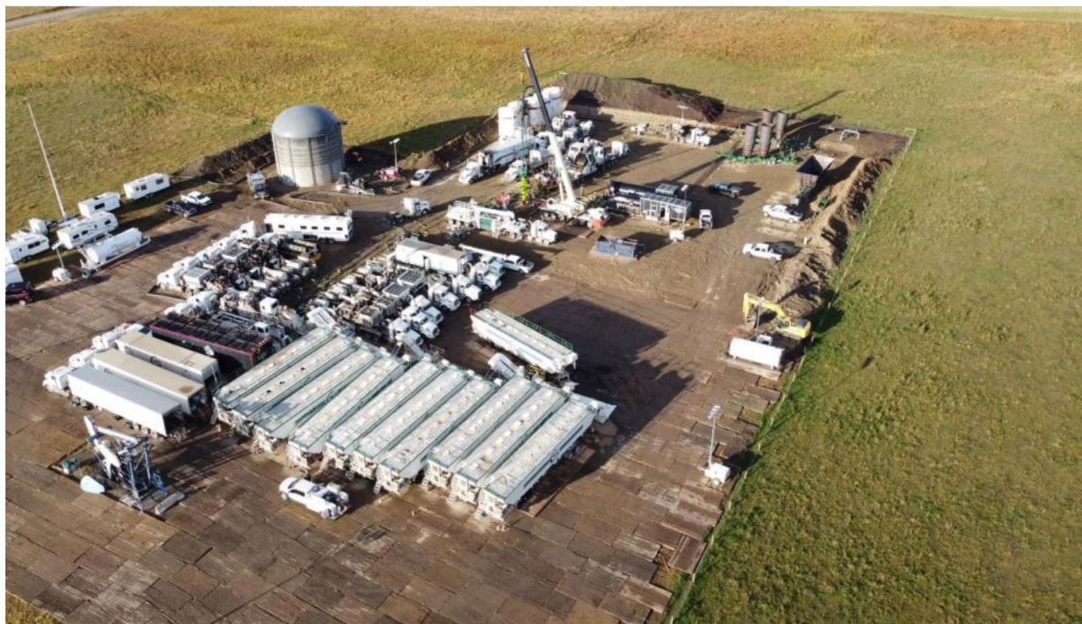
Figure 2. Aerial view of fracture spread on location at the Certus Caroline 1-27-33-05-W5 well.
