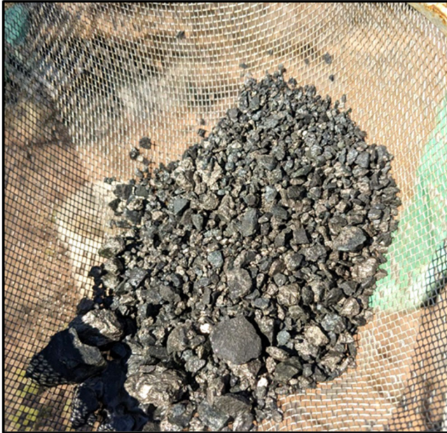
Figure 11 – Disseminated and matrix sulphides in RC drill chips (53m in NRC455)
