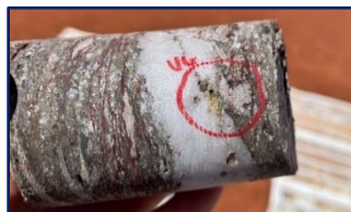
Plate 1: AHDD0018 (0.6 m @ 333 g/t Au from 20.2 m) – visible gold in quartz veins – HQ3 core
