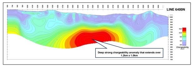
Figure 14. Cross-section of chargeability data from Line 6400N.
