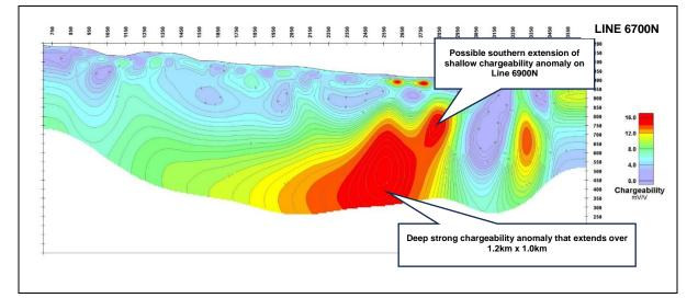
Figure 13. Cross-section of chargeability data from Line 6700N.
