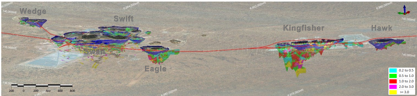
Figure 7: 3D view of Main Gidgee Mining Area looking down to the northeast. Free milling A$2,900 optimised pit shells (blue), MRE block models (coloured by Au g/t), existing pits (brown) and haul roads (red) over see-through satellite image.
