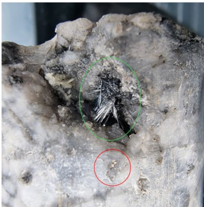
Figure 4 Acicular needle stibnite growths (green) in a late-stage vug in one of the quartz-carbonate breccias which also shows a cluster of native gold grains (red circle) just below the vug. (BKC015)
