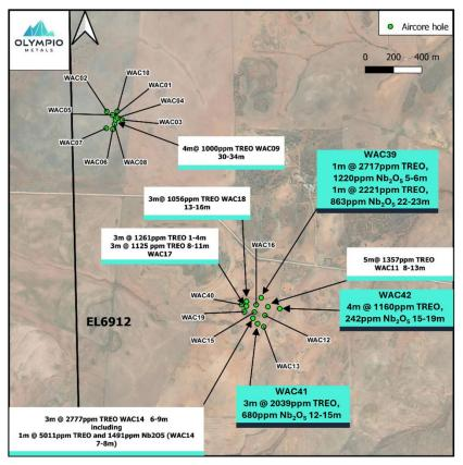
*Figure 3*: Collar locations of aircore drilling at W6 and W2 targets, Nov-Dec 2023.
