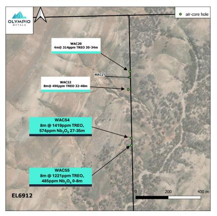
Figure 4: Collar locations of aircore drilling at W1 Carbonatite Target, Nov-Dec 2023
