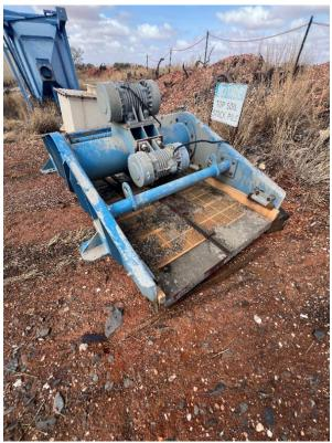
Figure 7 – Tailing Screen removed to replace the underpan
