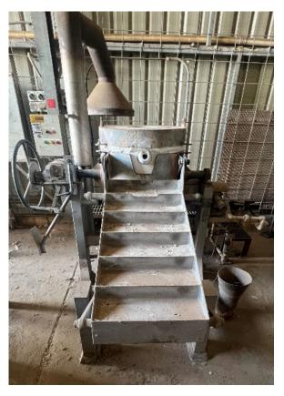
Figure 4 – Furnace replaced complete with new spout & crucible
