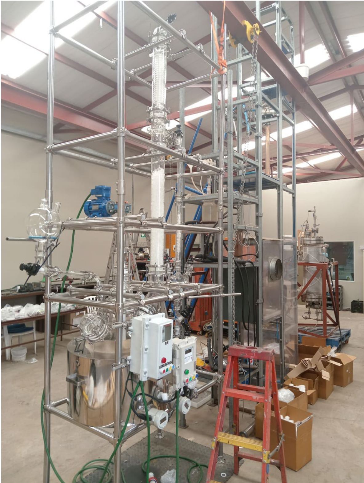
Image: Distillation column for Globe's Pilot Plant under construction at Resonant Group's facility in Johannesburg, South Africa.
