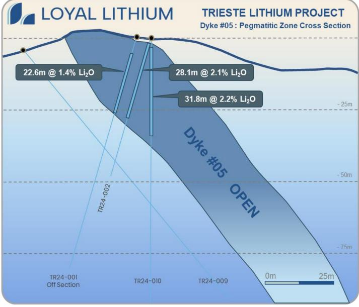
Figure 1: Trieste Lithium Project: Dyke #05 Cross section on section line A-A'.
