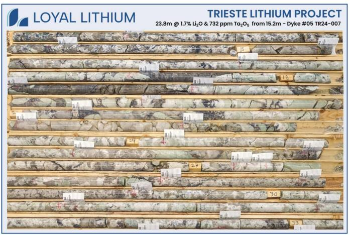
Appendix Image 9: Trieste Lithium Project – Dyke #05 core photo of Spodumene crystals drillhole TR24-007.
