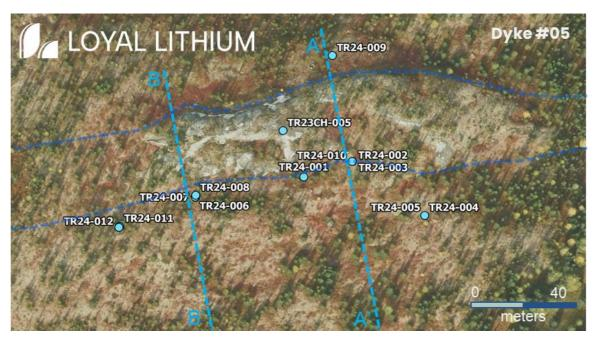
Appendix Image 1: Trieste Lithium Project - Dyke #05 plan showing drillhole locations and cross section lines.
