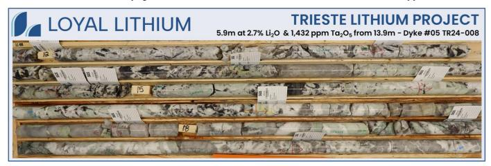
Appendix Image 8: Trieste Lithium Project – Dyke #05 core photo of a high grade lithium and tantalum interval from drillhole TR24-008.
