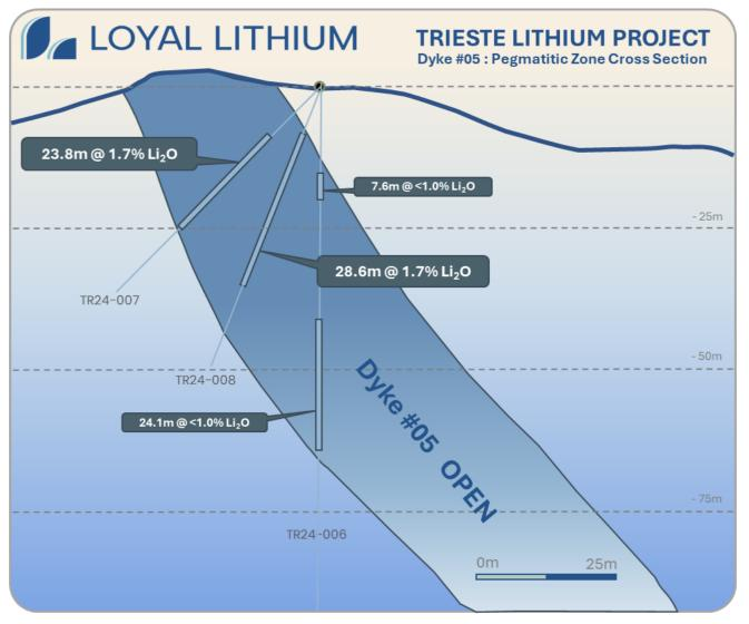
Appendix Image 7: Trieste Lithium Project - Dyke #05 cross section line B-B'. TR24-006 shown to illustrate an anomalous interval in pegmatite with extreme tantalum results of a maximum of 2,076ppm Ta<sub>2</sub>O<sub>5</sub>.
