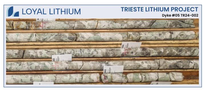
Appendix Image 6: Trieste Lithium Project - Zoomed in core photo of Spodumene crystals drillhole TR24-002.
