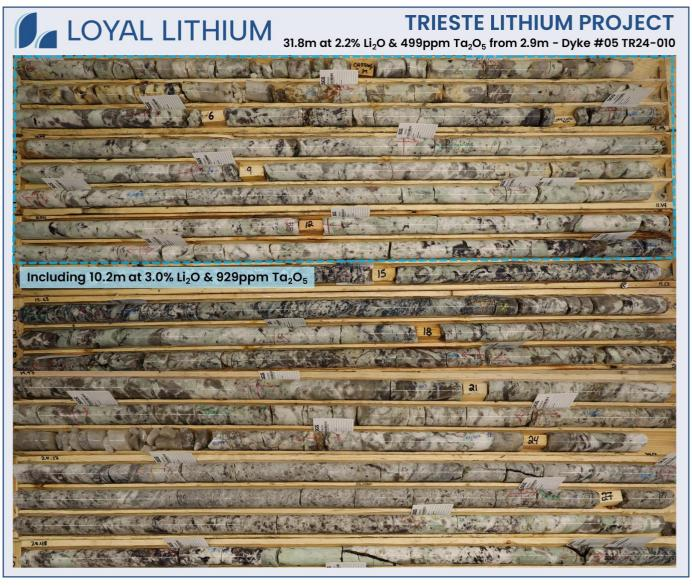
Appendix Image 3: Trieste Lithium Project - Dyke #05 core photo of Spodumene crystals drillhole TR24-010.
