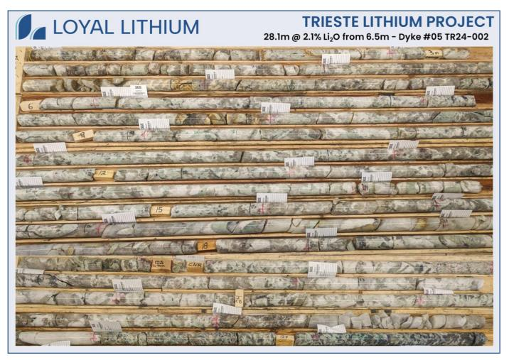
Appendix Image 5: Trieste Lithium Project - Zoomed in core photo of Spodumene crystals drillhole TR24-002.
