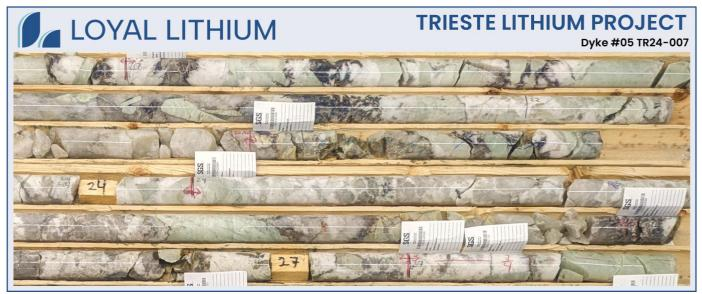
Appendix Image 10: Trieste Lithium Project - Dyke #05 core photo of Spodumene crystals drillhole TR24-007.
