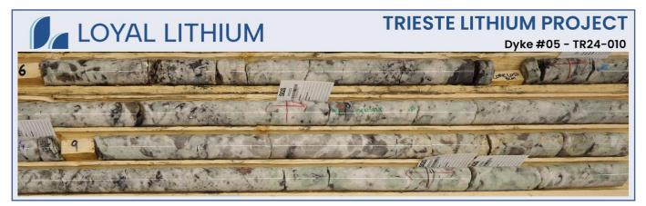
Appendix Image 4: Trieste Lithium Project - Zoomed in core photo of Spodumene crystals drillhole TR24-010.
