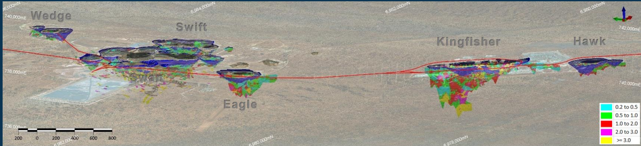
3D view of Main Gidgee Mining Area looking down to the northeast. Free milling A$2,900 optimised pit shells (blue), MRE block models (coloured by Au g/t), existing pits (brown) and haul roads (red) over see-through satellite image
