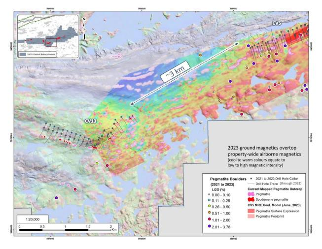
Figure 6: 2023 ground magnetic data presented atop property-wide airborne magnetic data, highlighting local trends along the CV5 to CV13 corridor (cool to colours = lows to high magnetic intensity).
