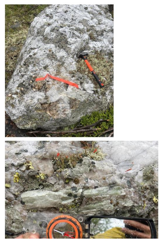
Figure 5: Top – spodumene pegmatite boulder situated ~2 km south of CV5, indicating potential for yet to be discovered spodumene pegmatite to the south and/or east of CV5's current known extent. Sample collected assayed 2.2%  $Li_2O$ . Bottom – spodumene crystal from same boulder.
