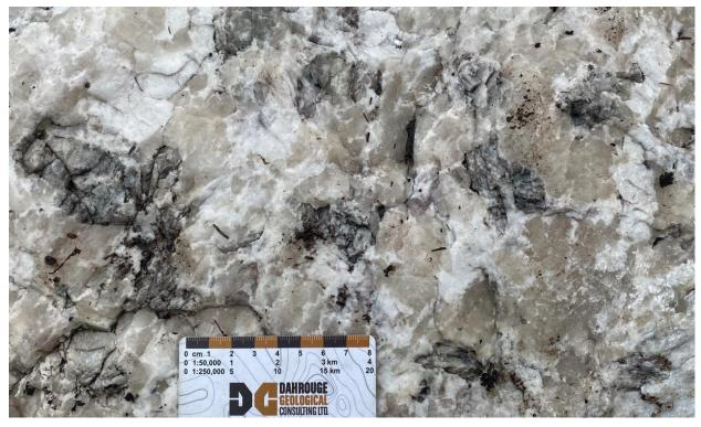
Figure 3: Spodumene crystals at CV14, a new spodumene pegmatite outcrop discovery in 2023, in a matrix of feldspar and smoky quartz.
