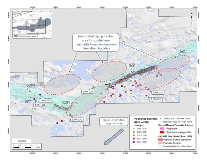
Figure 4: Interpreted high-potential areas for at or near-surface spodumene pegmatite based on downice mineralized boulders.
