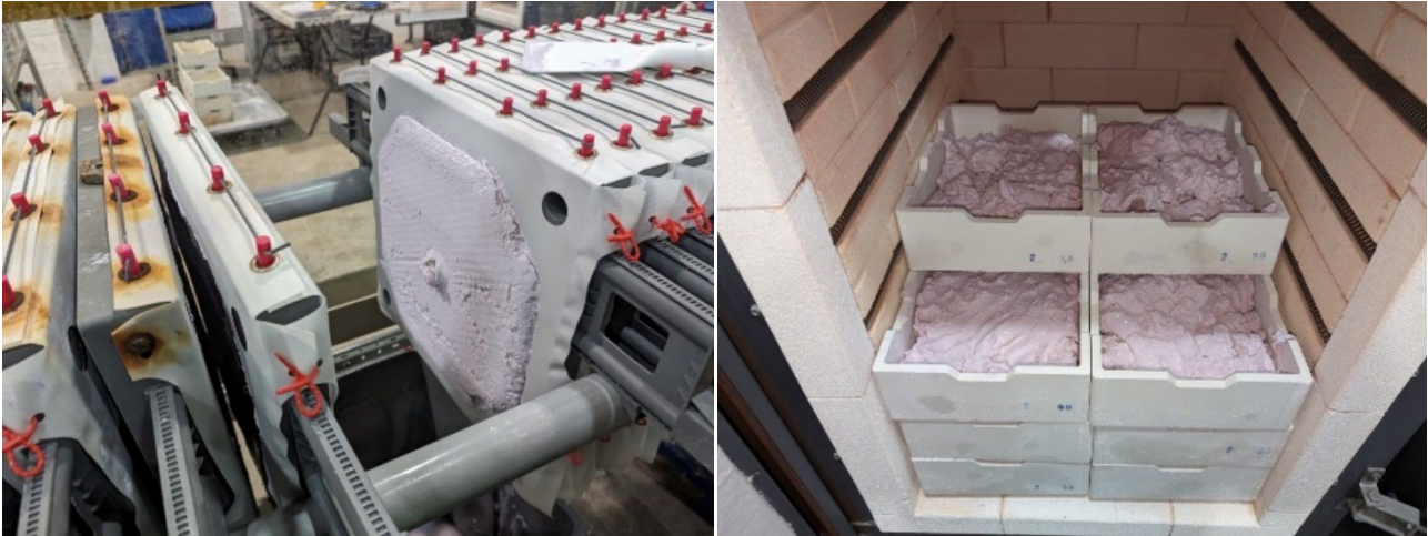
Figure 2: NdPr oxalate product produced post separation (left), and calcination feed (right).
