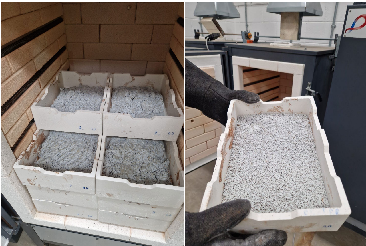
Figure 1: First NdPr oxide (>99.8% grade) production achieved from continuous operations at Ionic Technologies' Belfast Demonstration Plant.
