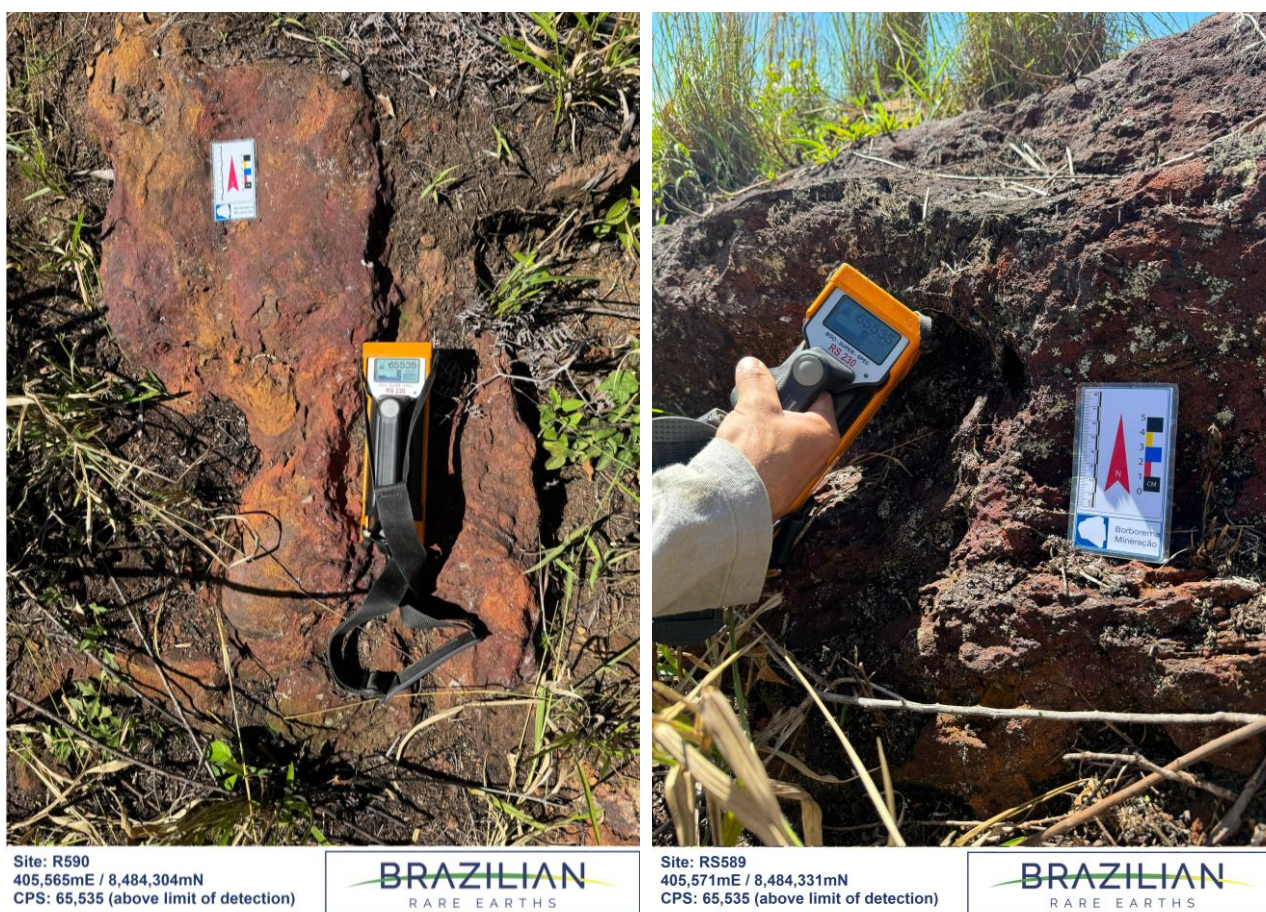
Figure 6: Pelé Target 1 outcrops - CPS values above the detection limit, indicative of Monte Alto style ultra-high grade REE-Nb-Sc mineralisation
