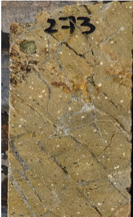
Gold Mineralisation (25.3 g/t Au) in Rhyolite at 272.3-273 m in LRCD152 (HQ Core)
