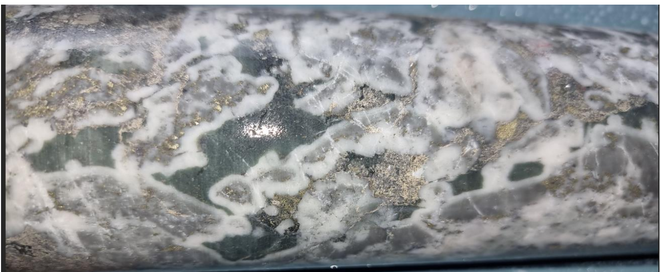
Figure 8 – Deep Mineralised Zone DRRCD0019 – Mineralisation styles and textures 374m to 399.1m down-hole. Upper Panel (field of view 0.27m) – Massive sphalerite(25%), quartz breccia(25%), galena(50%). Lower Panel (Field of view 16cm) – Chalcedonic vein textures with interstitial Chalcopryite (2%-3%), pyrite (3%-5%).
