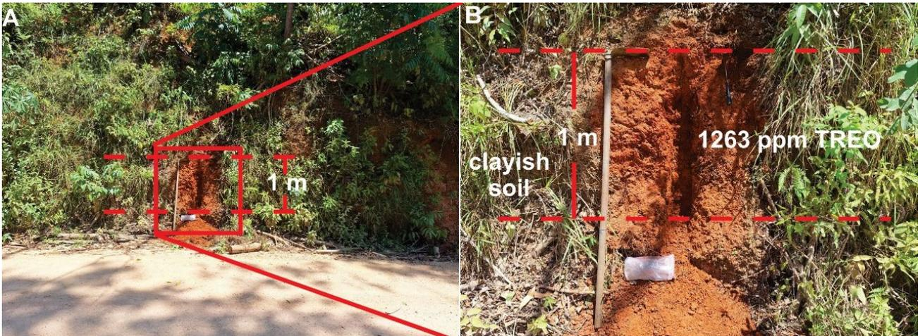
Figure 3: Surface Channel Sampling EQ-CG-562 at the Rio Negro Target.
