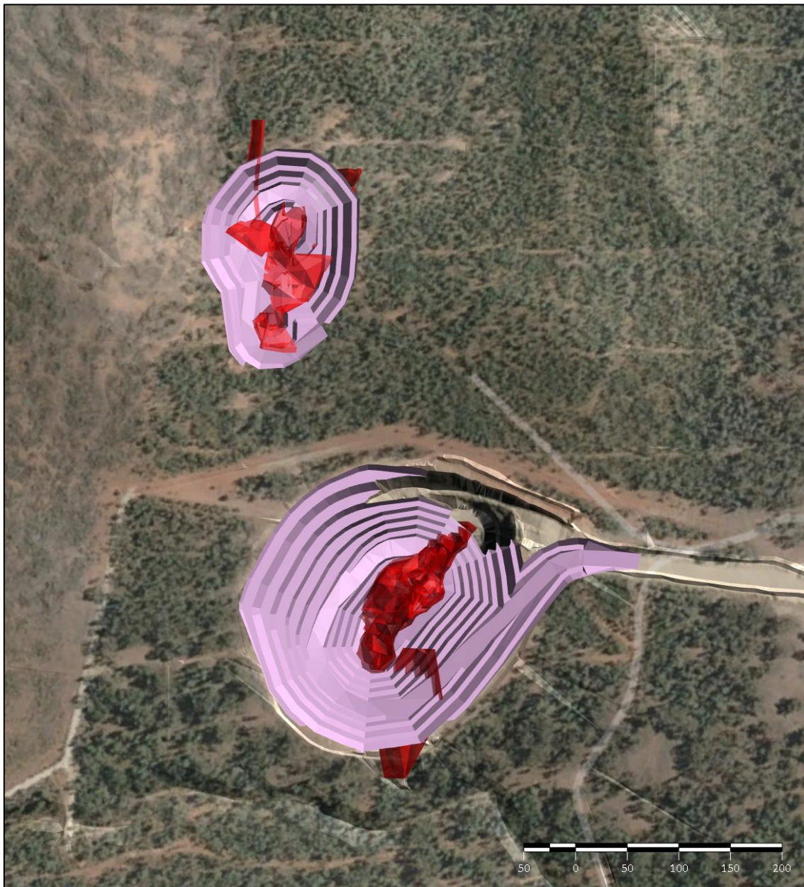
Figure 2: Open pit mine designs for Pearse North and South.
