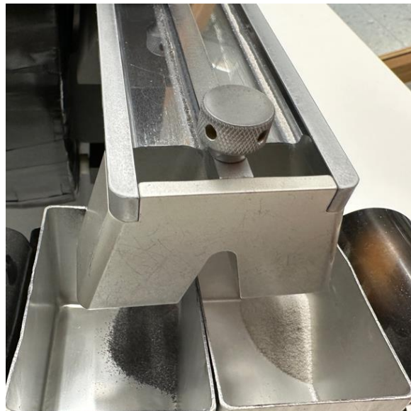
Figure 1: Dry magnetic separation on sample KUSGS37 showing magnetic concentrate on the left (black) and non-magnetic residual material on the right (light grey).
