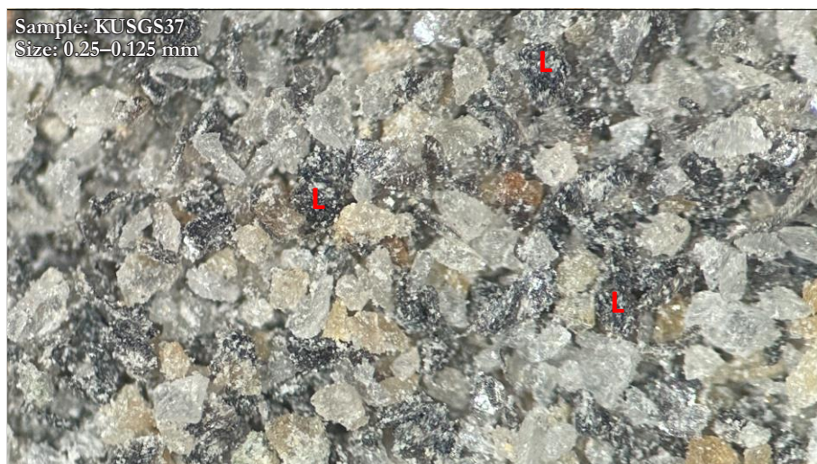
Figure 2. Microphotograph of sample KUSGS37 sieved fraction 0.25–0.125 mm. Nearly all black lithium mica crystals (L) are fully liberated.
