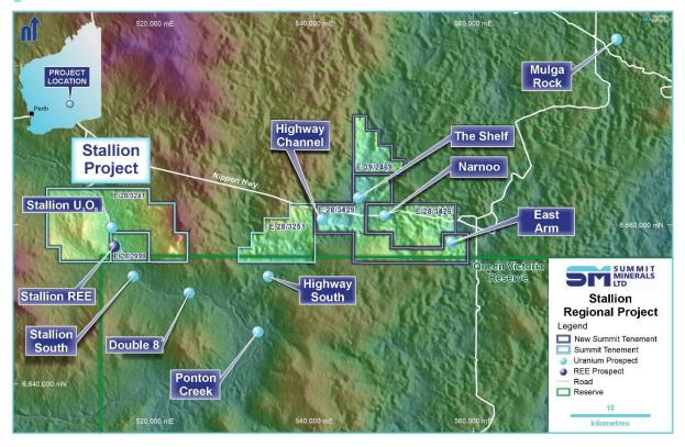
Figure 1 - Summit controls 442 km<sup>2</sup> of exploration tenements and applications underlain by Tertiary palaeochannels at Stallion. These palaeochannels are known to host several uranium deposits and drilled uranium prospects, including the 3.2Mlb Stallion uranium resource.
