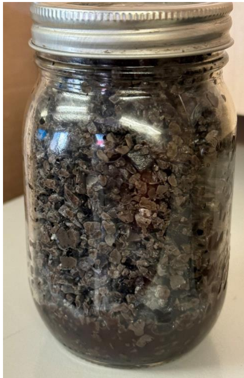
Figure 1: The drill cuttings from a shallow Clastic horizon at Bosydaba#1 well showing the same lithological units as those that are logged at the Paradox Project.
