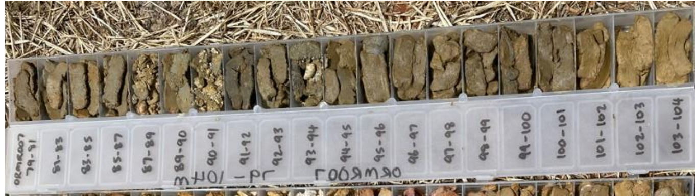
Drill samples from ORMR007 at the Rankin Rd Target showing the limonite rich fluid from 101-104m with a small uranium zone occurring at 101m. The kaolinitic clay marker bed at 85-94m.
