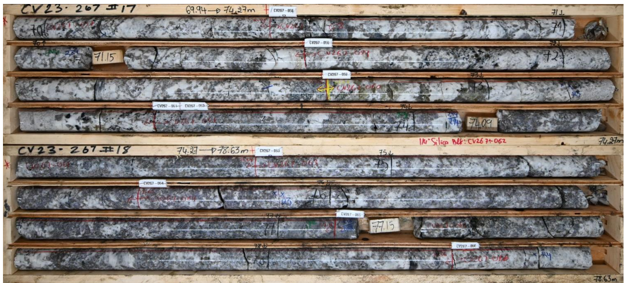
Figure 8: Spodumene pegmatite from drill hole CV23-267. Approximately 1.0% Li 2 O over interval (70.0 m to 78.6 m)
