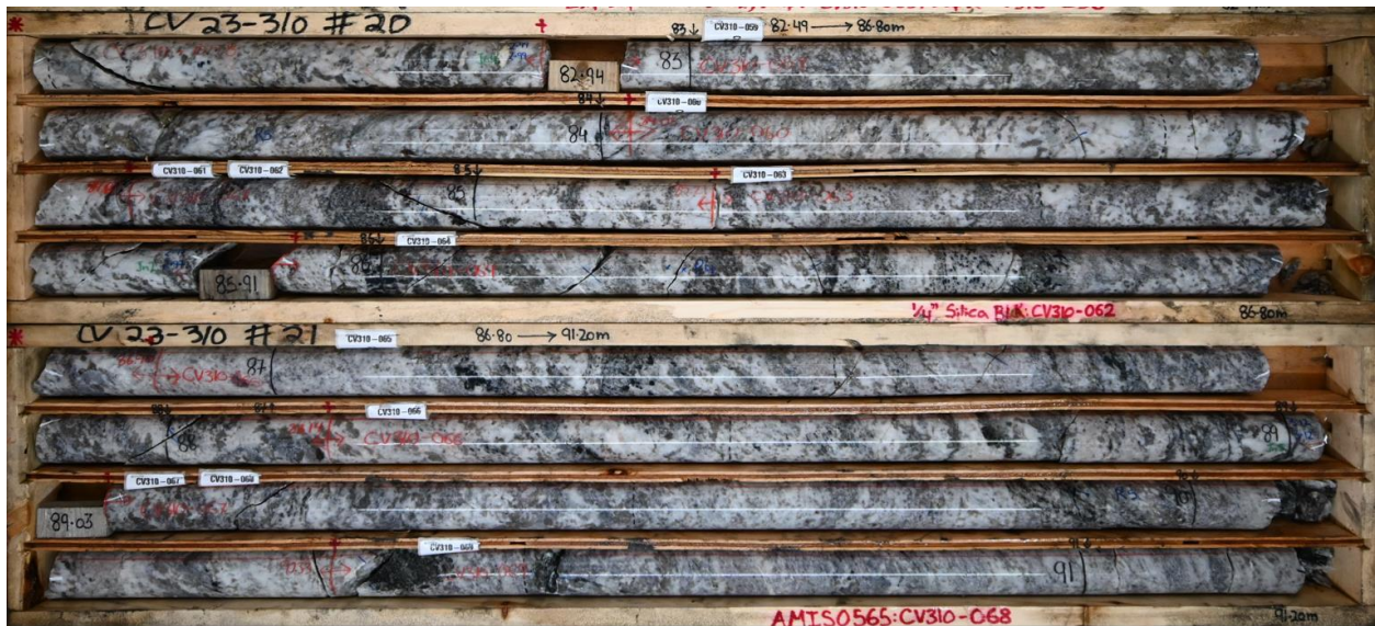
Figure 9: Spodumene pegmatite from drill hole CV23-310. Approximately 1.0% \text{Li}_2\text{O} over interval (82.5 m to 91.2 m)
