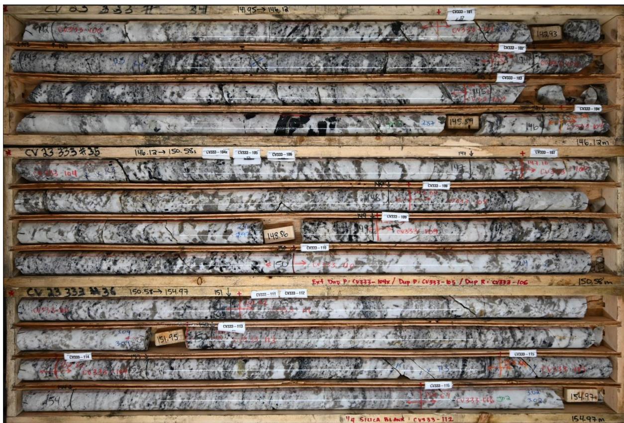
Figure 10: Spodumene pegmatite from drill hole CV23-333, including 7.7 m at 1.35% \text{Li}_2\text{O} (146.0 m to 153.7 m)
