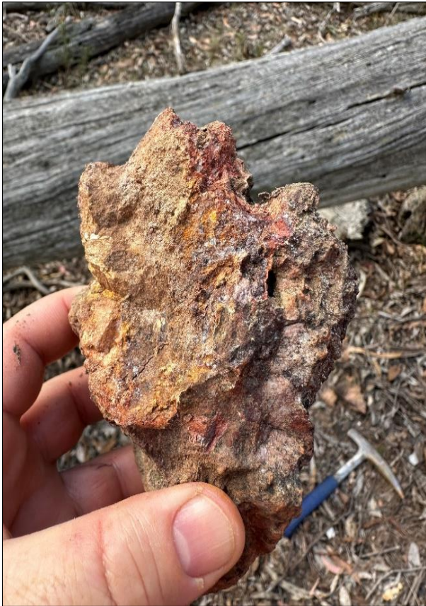
Figure 5 – Silver-Base Metal mineralisation within gossanous siltstone yielding 80.9 g/t Ag, 0.1% Cu, 0.4% Pb & 0.12% Zn, 0.51% Ba 3000287 from sample 3000551
