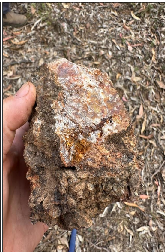
Figure 4 – Silver mineralisation within ferruginous quartz yielding 183 g/t Ag, 970 ppm Ba from sample 3000551
