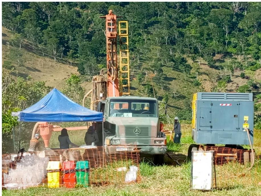
*Figure 2 – RC drill rig drilling at the Rio Negro prospect.*
