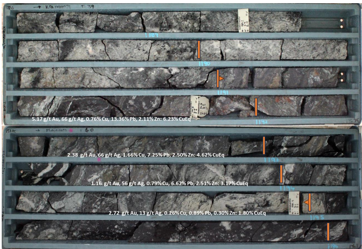
Figure 2: Drill core from KSNDDH021 (4m wide sulphide rich breccia lode (estimated true width of 2m) within a broader 31.6m wide brecciated and veined lode zone from 175.3mdh).
