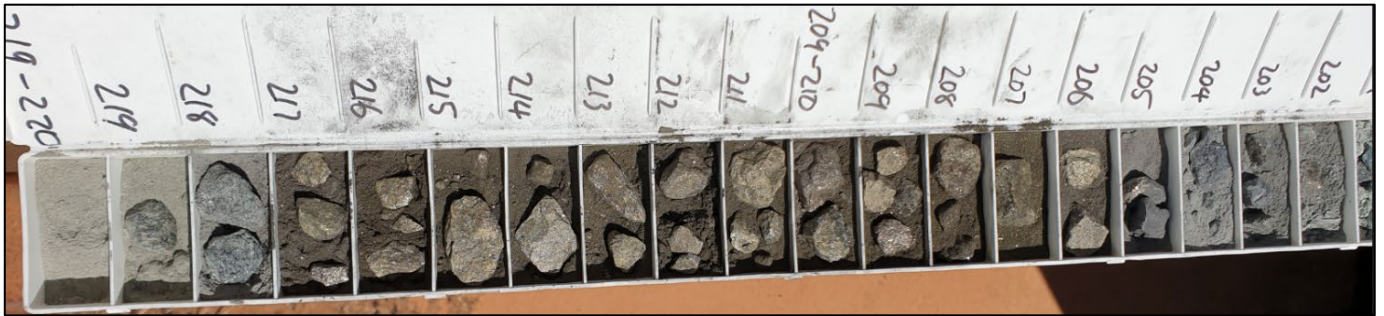
Figure 2: Chip tray showing massive sulphide copper-zinc mineralisation in 22AER005B
