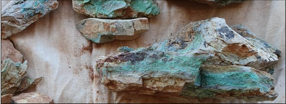
Photo 1. Rock chip sample KB03113, which returned 15.3% Copper 2 , comprised of oxidized white meta-tuffaceous siltstone with oxide copper mineralisation (green/dark grey in photo).
