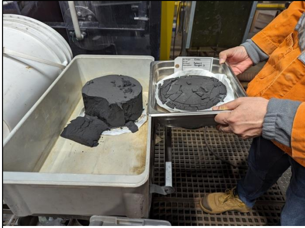
Figure 18: Dried DR concentrate (L) and RF concentrate (R) after batch reverse flotation
