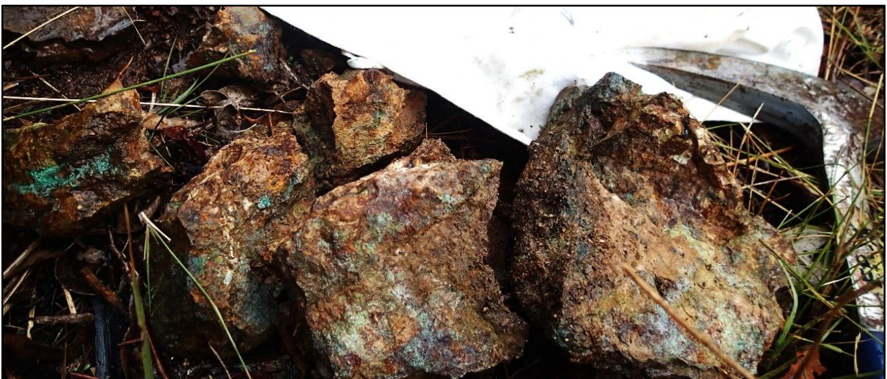
Figure 1: Sample R1026: 1.235g/t Au, 39.1g/t Ag, 10.45% Cu, 331ppm La, 45.3ppm Mo, 4850ppm Pb & 19.6ppm Sn
