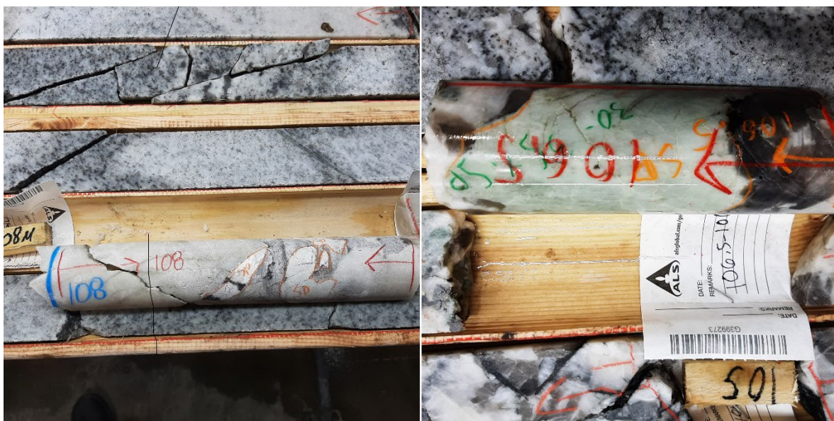
Figure 2: Spodumene crystals evident in CAD56 drill core Dyke B106.5-106.8m 2.31% Li 2 O and 108.15-108.4m 0.60% Li 2 O, (see Table 1 )
