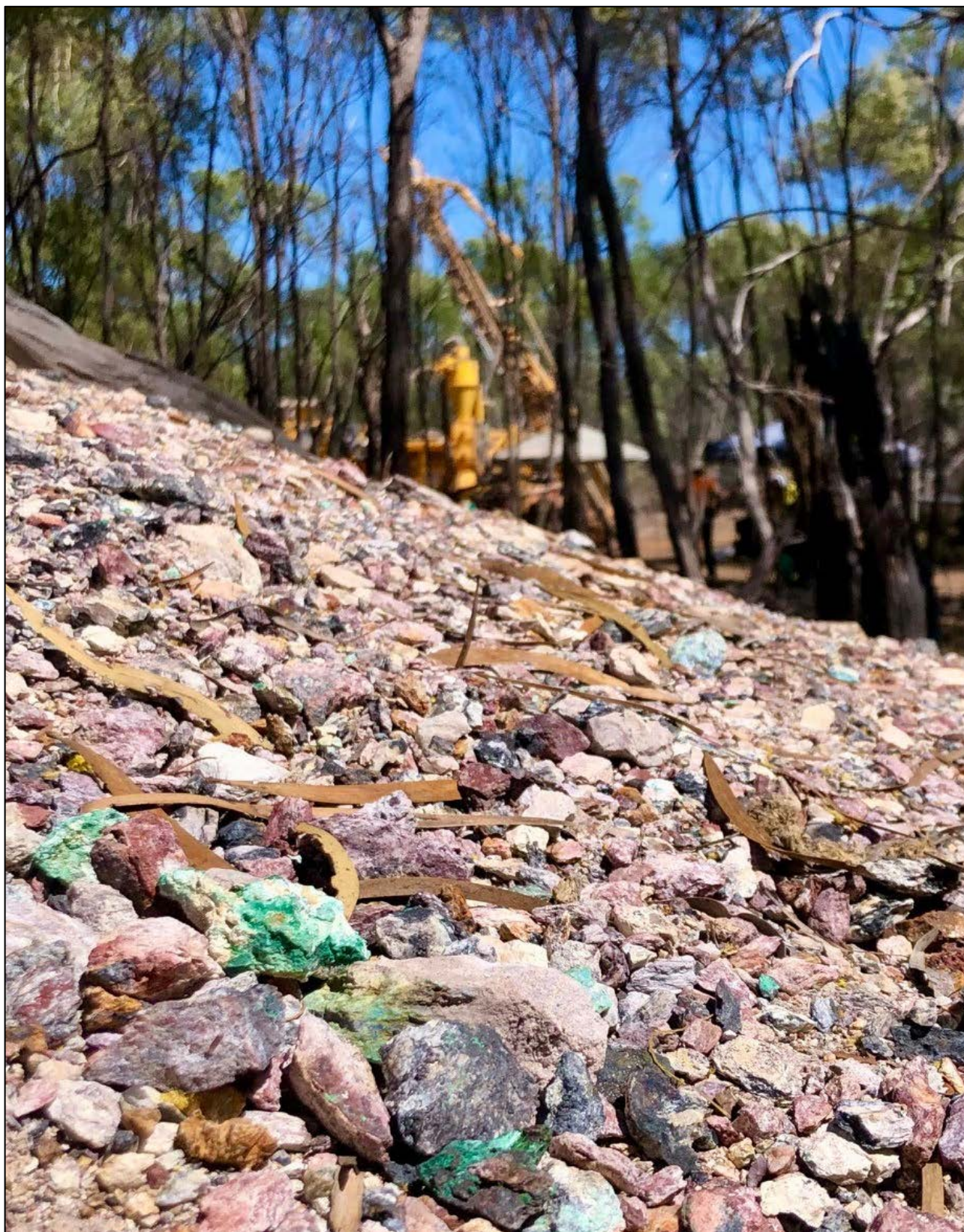
Figure 3: View of RC drill rig over spoils pile adjacent to the Sapidinus Shaft. Green malachite (copper carbonate) can be seen within the pile amongst weathered pumice breccia.
