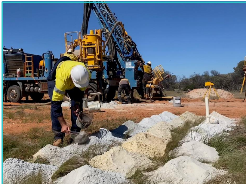
Photo 1: Maiden Lithium drill hole IVRC028 drilling and sampling in progress.
