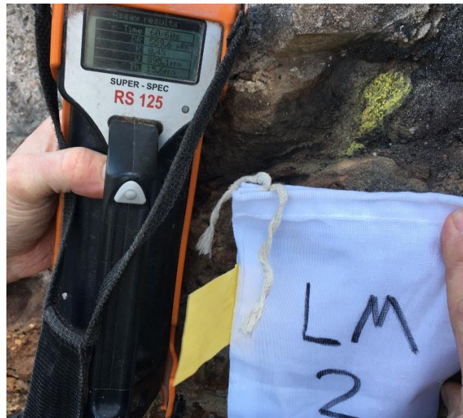
Figure 4. Carnotite in dark-coloured beds bounded by sandstone (sample LM2)
