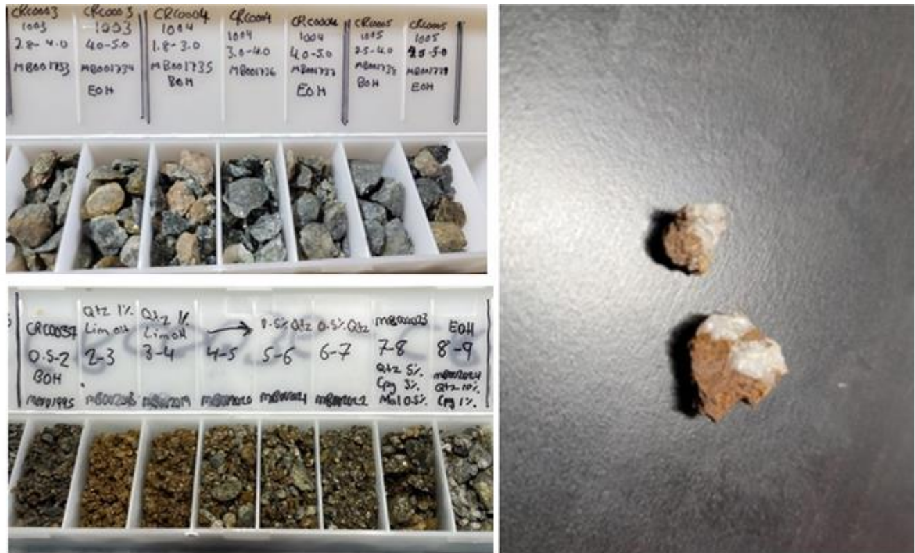
FIGURE 2: SELECTED BOTTOM OF HOLE SAMPLES FROM THE O-2 TARGET. CHIP TRAY SAMPLES ON LEFT AND ANKERITE-QUARTZ VEIN ALTERATION ON RIGHT TARGET
