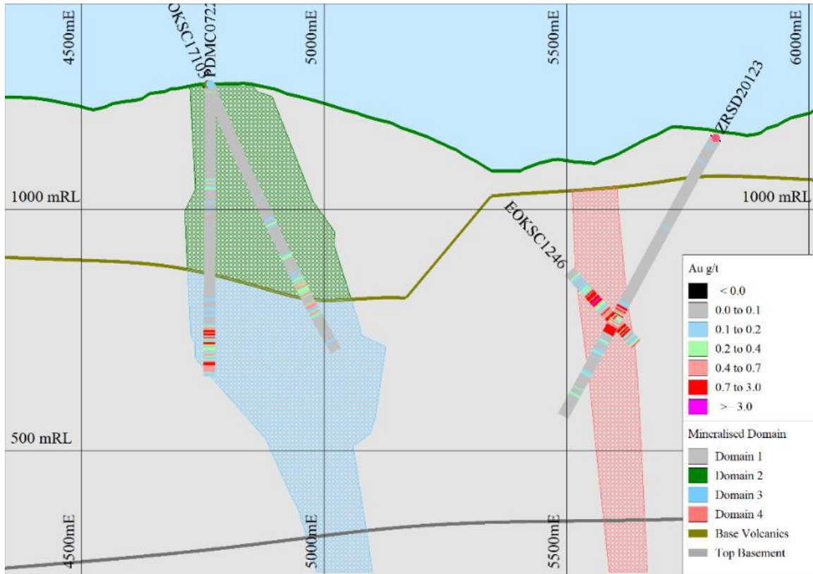
Figure 12: Shanac mineralisation domains, cross section 10,065 mN, looking north
