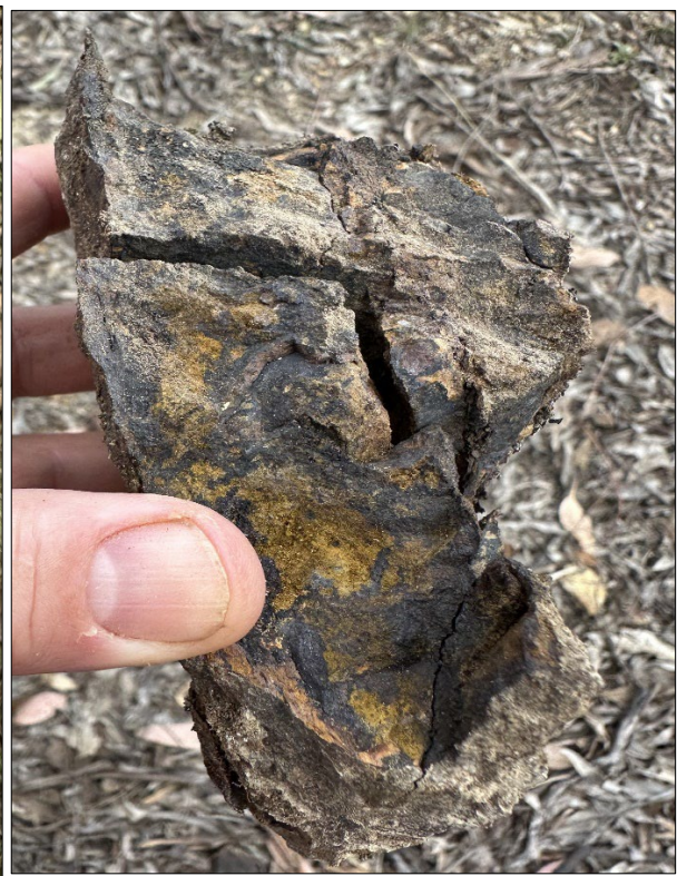
Figure 6 – Golden Wattle Gold mineralisation within gossan yielding 11.45 g/t Au, 0.97 g/t Ag, 1,695 ppm Pb, 720 ppm Ba from sample 3000491
