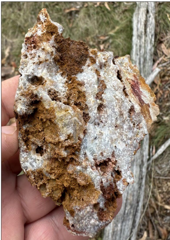
Figure 2 – Henry Zone hosting gold-silver mineralisation within weathered chert with oxidised sulphide clast yielding 2.31 g/t Au, 3.31 Ag from sample 3000411
