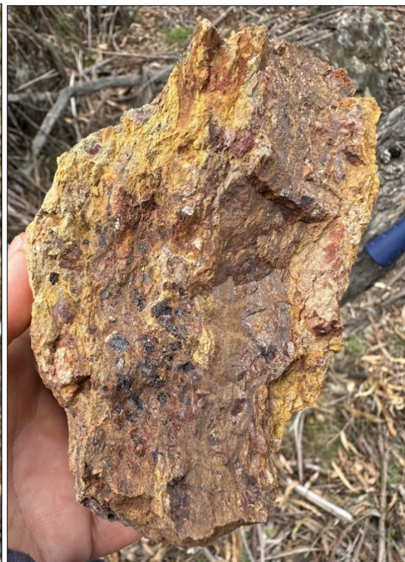
Figure 3 – Henry Zone hosting gold-silver mineralisation within gossan yielding 3.76 g/t Au, 2.83 g/t Ag, 510 ppm Ba from sample 3000415
