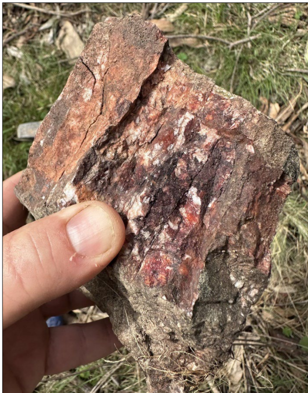
Figure 5 – Golden Wattle Gold mineralisation within ferruginous quartz yielding 23 g/t Au, from sample 3000503
