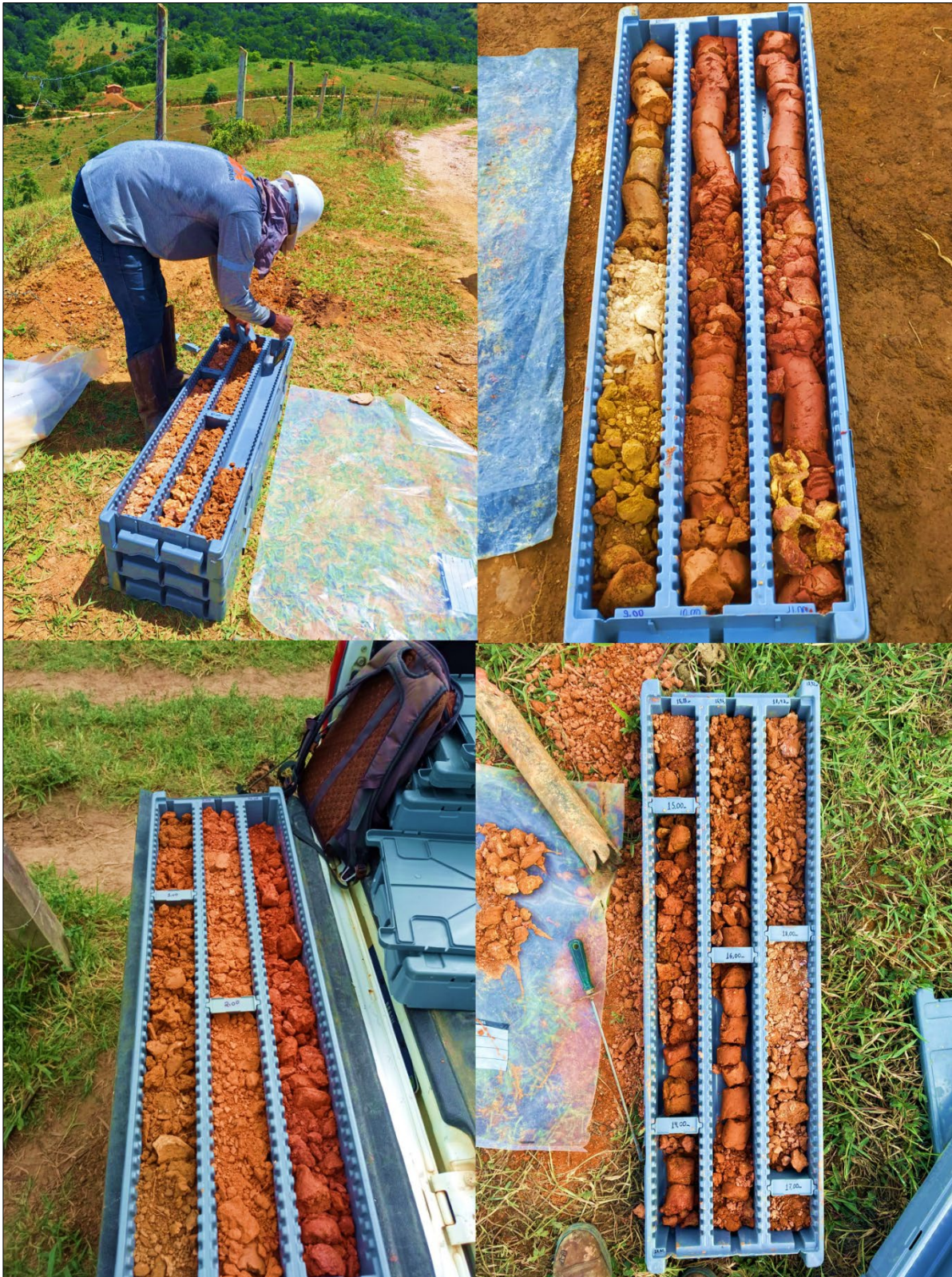
Figure 9: Material intercepted by auger drilling stored in plastic core cases in the field to be transported to the exploration shed.
