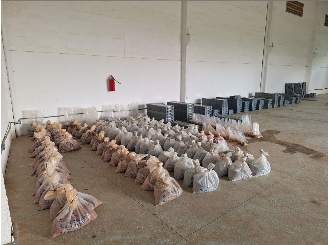
Figure 10: Plastic core cases with auger drilling samples and plastic bags with RC drilling samples stored in the Equinox exploration shed in Jequié.
