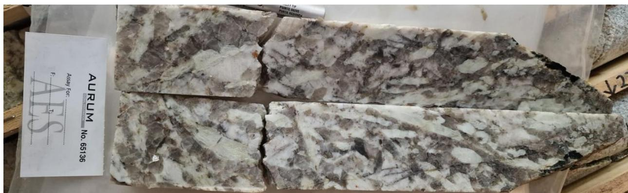
Figure 7: **Spodumene pegmatite in drill core DDH 23-1597-02**
