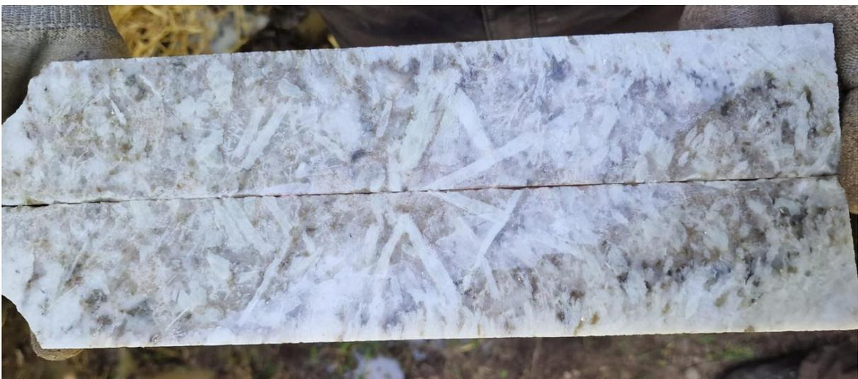
Figure 6: Spodumene pegmatite in drill core DDH 23-1597-01 (PEG-01 [part of]; 34.59-34.94. Sample AES65107 reporting intercept apparent thickness of 0.36m \ True thickness 0.05m @ 2.95% Li<sub>2</sub>O)
