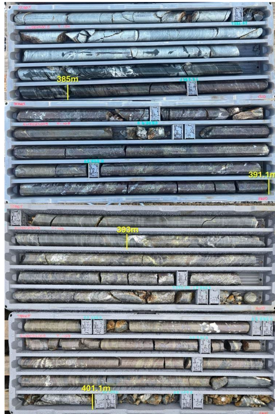
Figure 3 - Massive Zn and Cu Mineralisation in EWDD24005
